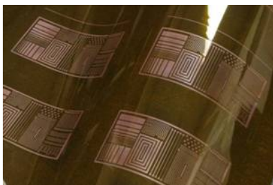
Figure 8. Inkjetted copper ink printed on flexible substrate
