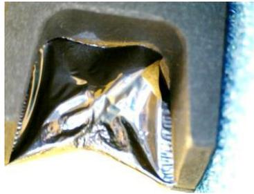
Fig. 4. Picture of damaged graphene foil.
