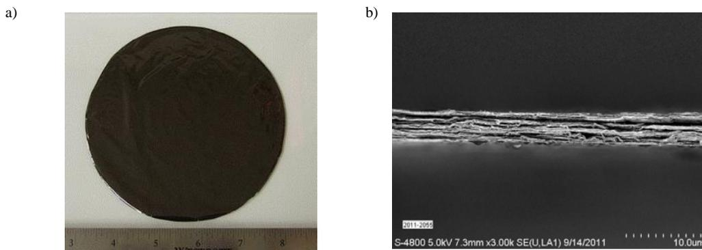
Fig. 1. Images of graphene foils: a) a photograph of a fabricated foil, scale in inches; b) SEM of graphene foil cross section (scale on image). The dimensions of a graphene stripper foil on the carousel of Eclipse cyclotrons is 10mm x 10mm.
